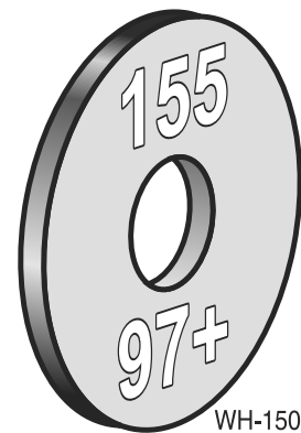
Figure 11 Propane gas orifice identification WM97+155
